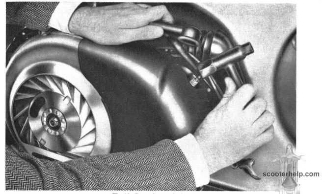
Fig. 14—Removing spark-plug
